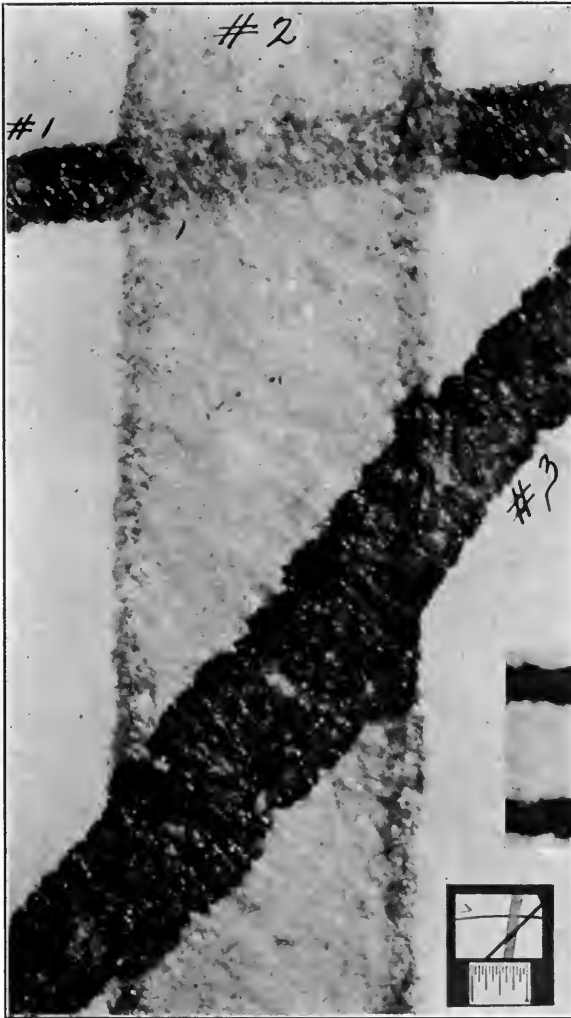
FIG. 160—The order of writing of three lines shown clearly by enlarged photograph. Line No. 2 was blotted at once and No. 3 was made before No. 2 was entirely dry.
